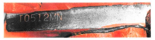
Above: Photograph of the engine pad on this COPO 427 Camaro. Note the machine grooves or marks on the deck surface. This engine pad has been decked and restamped with new numbers which are not authentic to this block. The original broach marks are also gone now that the deck was machined and restamped.
